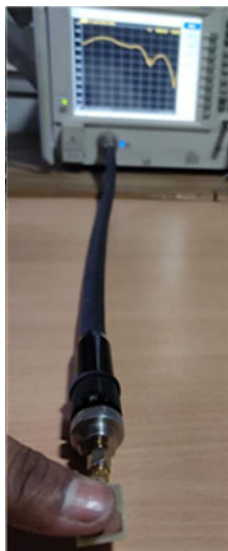
Figure 24. Measurement setup for glucose level monitoring by loading of thumb on radiating patch.
