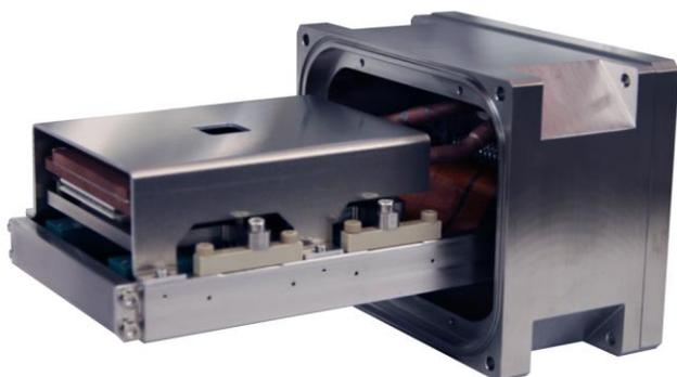
**Figure 1.** The pnCCD camera for TEM applications.
