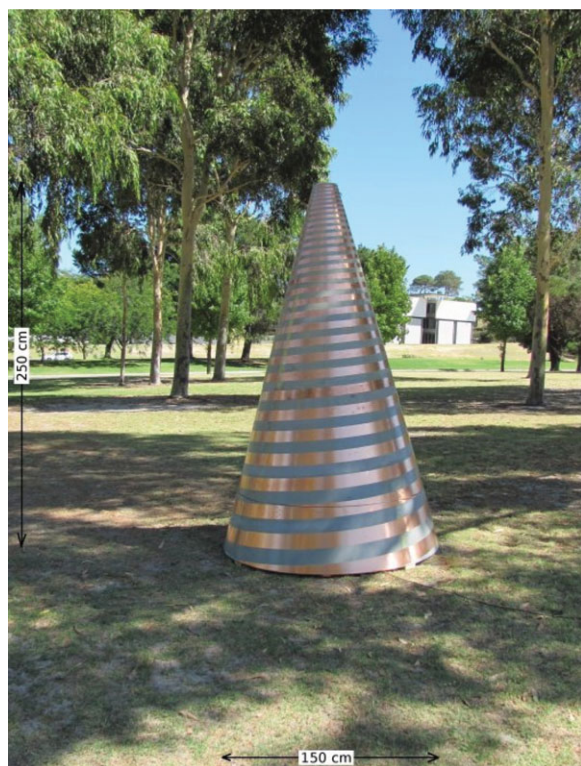
Figure 26. The conical log spiral antenna (before painting) during tests at Curtin University.
