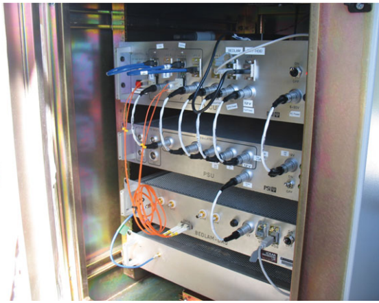
Figure 5. The RF-shielded rack housing BIGHORNS back-end components (from the bottom to top : box with a second gain stage and RF-filters; BEDLAM spectrometer; power unit; and PC computer unit).
