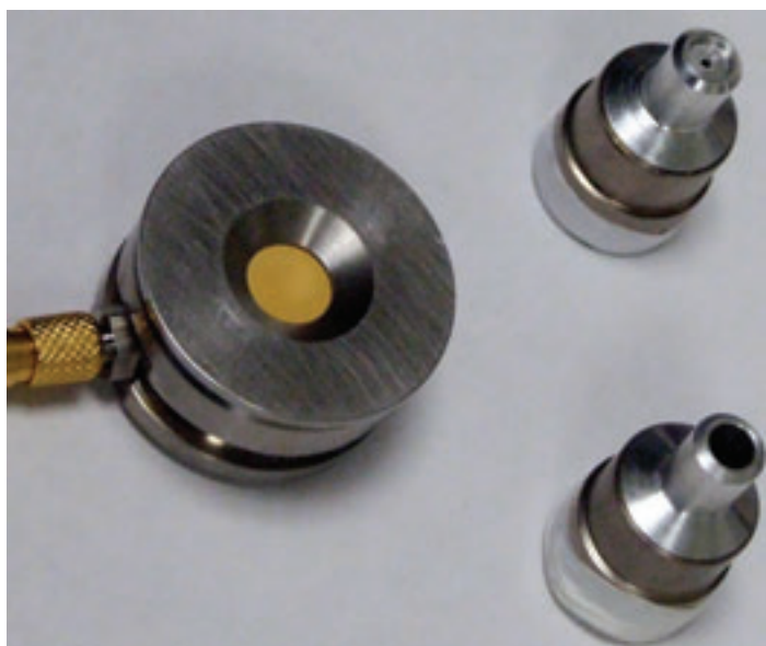
Figure 6: Quartz crystal thickness meter (left) and Oxford Instruments collimator with (top right) and without insert (bottom right). Teflon tape has been placed around the base of the collimators.
