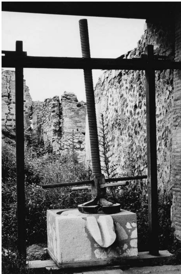
Figure 4.27 Reconstructed vertical oil press at Pompeii, VII.7.
