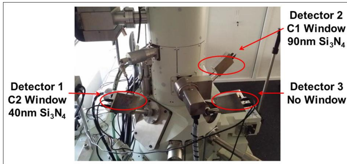
Figure 1. JEOL 7001F FEGSEM with multiple Amptek SDD's operating with a Moran Scientific Microanalysis and X-ray Mapping system.
