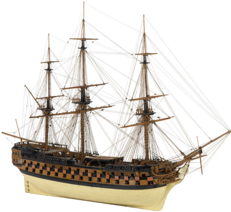
Figure 1. This model depicts the third-rate ship of the line HMS Mars , which took part in the Spithead mutiny. Its basic layout is typical of the warships involved in the 1797 fleet mutinies. The quarterdeck is visible between the two rear masts, while the forecabin is the area forward of the ship's boats stowed in the centre of the model. The raised platform aft of the quarterdeck is the poop deck, with the captain's great cabin located directly below it, accessed from the quarterdeck. National Maritime Museum, Greenwich, London, Royal United Service Institution Collection. Object ID: SLR0577.
