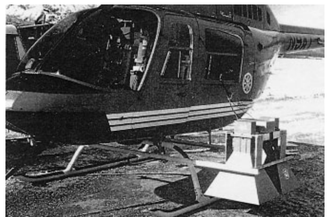
Fig. 3. The FM-CW radar system mounted to a Bell Jet Ranger 206B helicopter. Receiver components are mounted in a small box between the antennas. A coaxial cable from the helicopter window feeds power to the transmitter.
