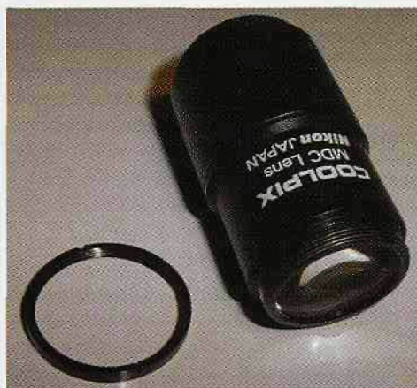
Picture 2: (Left) Nikon MDC relay lens (part number 82014). The small ring located on the left side of this picture had to be removed. The field of view (or field number) of this lens is 18 mm.
