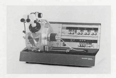
**RES 010** - state-of-the-art, high speed ion beam deposition system for the finest grain films. New generation ion beam milling machine with fast, true topographic milling of inhomogeneous materials.
