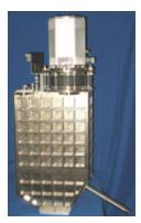
Microcalorimetry energydispersive X-ray spectrometry (Microcal EDS) offers the same qualitative and quantitative analysis capabilities as conventional EDS but with better spatial resolution because improved energy resolution allows analysis at low electron beam energies. The Microcal EDS consists of a thin Bi X-ray absorber in thermal contact with a superconducting transition-edge
