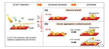
Figure 1. Schematic of the mechanism of copper cluster formation and growth at the solid-liquid interface under (a) low and (b) high photoreduction rate. The growth of the copper cluster into a final shape can be influenced by viscosity at the interface.
