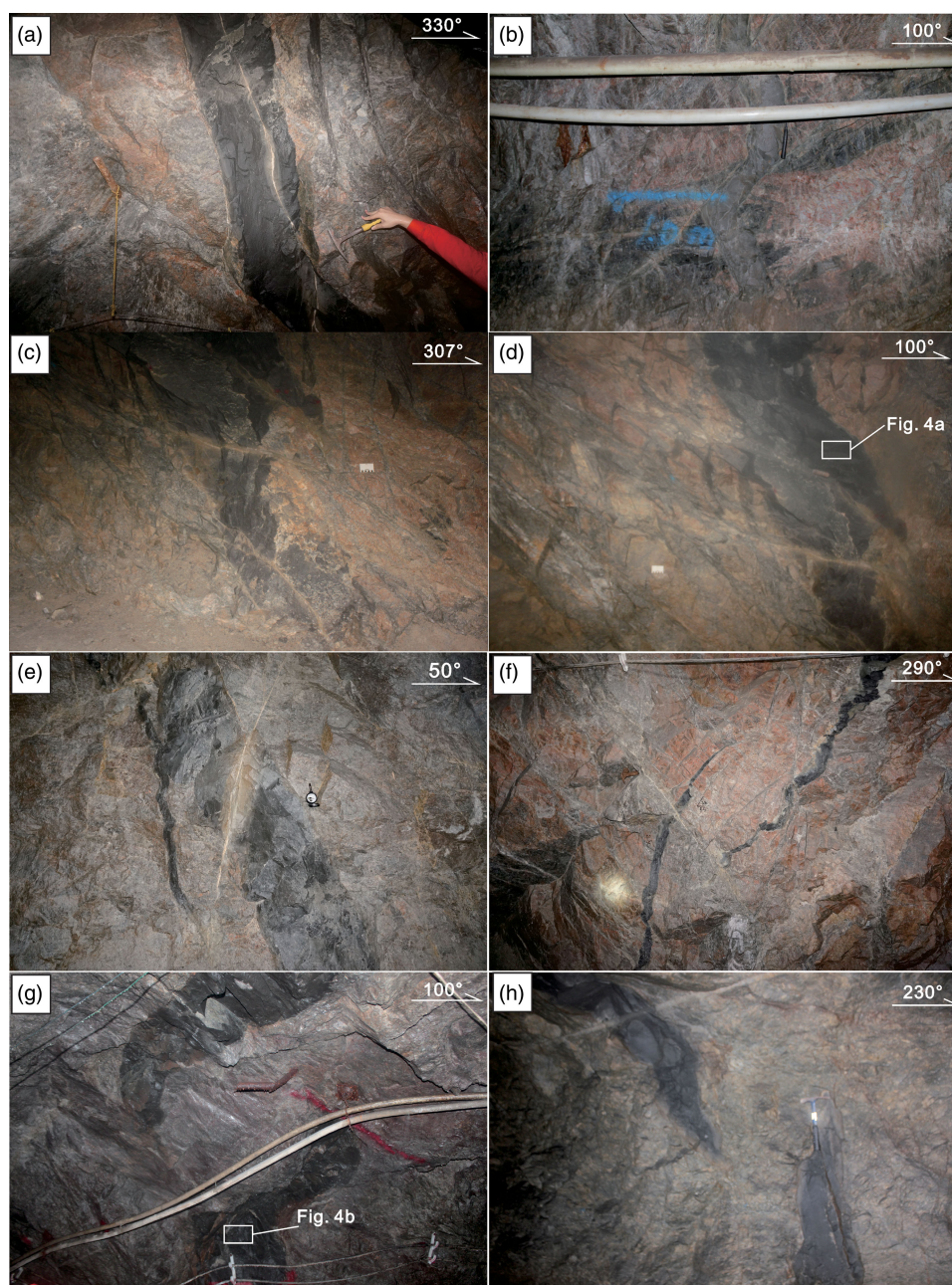
Fig. 3. (Colour online) Field photographs of the lamprophyre dikes in the Sizhuang gold deposit. (a) WNW-striking steep-dipping lamprophyre dike, with sharp straight contacts and (b) NNW-SSE-striking continuous dike segments, with non-overlapping and zigzag morphologies, in the K-feldspar altered granites. (c) NNE-SSW-striking dike segments with non-overlapping morphologies and horns beyond the offset step. (d) NNE-SSW-striking dike with small stepping continuous offsets in the K-feldspar altered granites. Note the localized dike-normal quartz veins near the stepovers in (c) and (d). (e) NNW-striking continuous dike segments with small stepping offset and horn beyond the offset step in the sericite-quartz altered granites. Note the quartz vein cutting through the step segment sharply. (f) NNE-SSW-striking discontinuous dike segments with lower-stepping overlapping offsets in the K-feldspar altered granites. Note the dike-normal quartz veins restricted to rock-bridge zone. (g) NNE-striking discontinuous dike segments with upper-stepping non-overlapping offsets in the sericite-quartz altered granites. Note the slight curvatures around dike tips. (h) NW-SE-striking discontinuous dike segments with lower-stepping non-overlapping offsets in the sericite-quartz altered granites. Note the slight curvature in the internal part and the thin apophyse in the outer part around dike tips.
