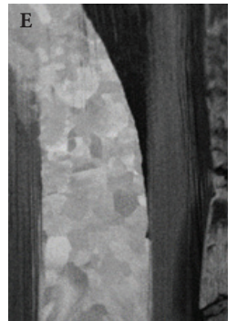
Correlative 3D-workflow: A) Hall sensor with internal defects, B) X-ray 3D image to localize bond wires and connections, C) Open sample with massive ablation laser and release Region of Interest, D) Fine polishing of defect structure using focused ion beam, E) HR imaging of defective area
