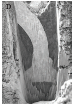
Correlative 3D-workflow: A) Hall sensor with internal defects, B) X-ray 3D image to localize bond wires and connections, C) Open sample with massive ablation laser and release Region of Interest, D) Fine polishing of defect structure using focused ion beam, E) HR imaging of defective area
