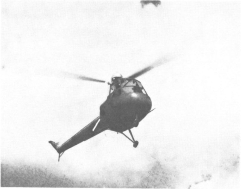
Saunders-Roe Skeeter fitted with Napier rocket booster system gives outstanding vertical flight performance for operations at altitude and in the tropics
