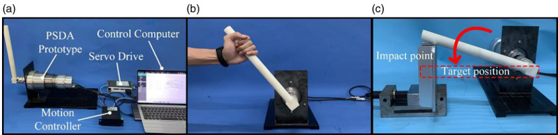
Figure 15. PSDA experiments (a) the experiment setup, (b) damping experiment, (c) impact experiment.
