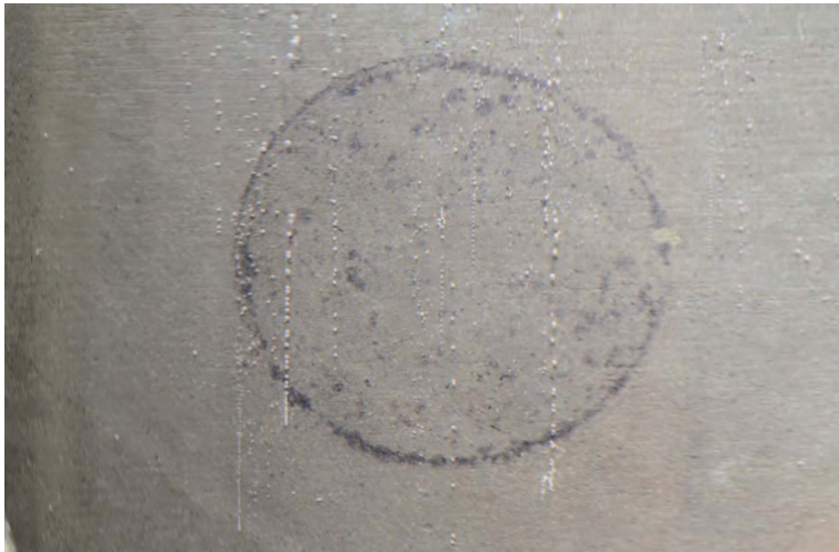
FIG. 8. Photograph showing the discharge of gas from the injection face of sample COx-1, following submersion in glycerol and gentle heating (the imprint of the central filter disc is clearly visible in the photo). The discharge of gas was both localized and often episodic, with discrete streams of gas bubbles released following a quiescent periods of inactivity.
