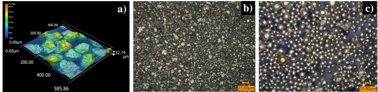
Figure 1. Micrographs of a) H13 powder milled at 50 minutes and visualized in 3D optic microscopy, b) H13 obtained at 120 minutes by mechanical alloyed and c) commercial powder alloy H13.
