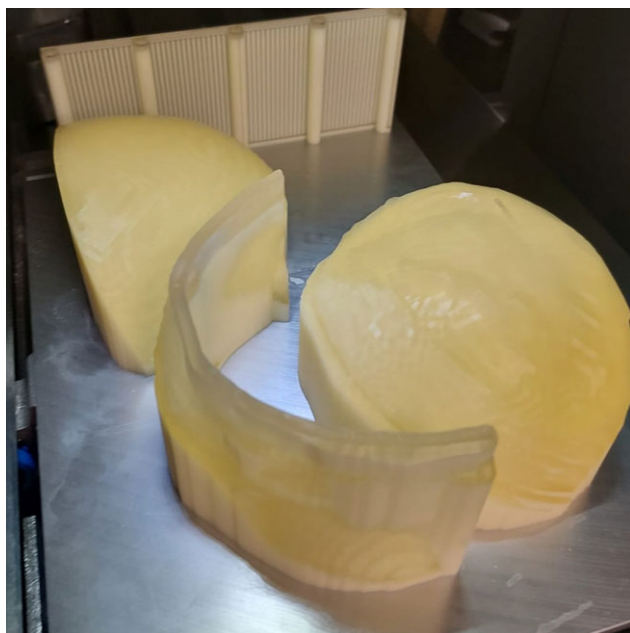
Figure 2. The figure above shows a 3D-printed model of the patient's head, divided into three parts. These must be post-processed to remove support material (wax) by dissolving it in hot vegetable oil. After post-processing, they can be assembled by auto-generated male-female plugs and super glue.
