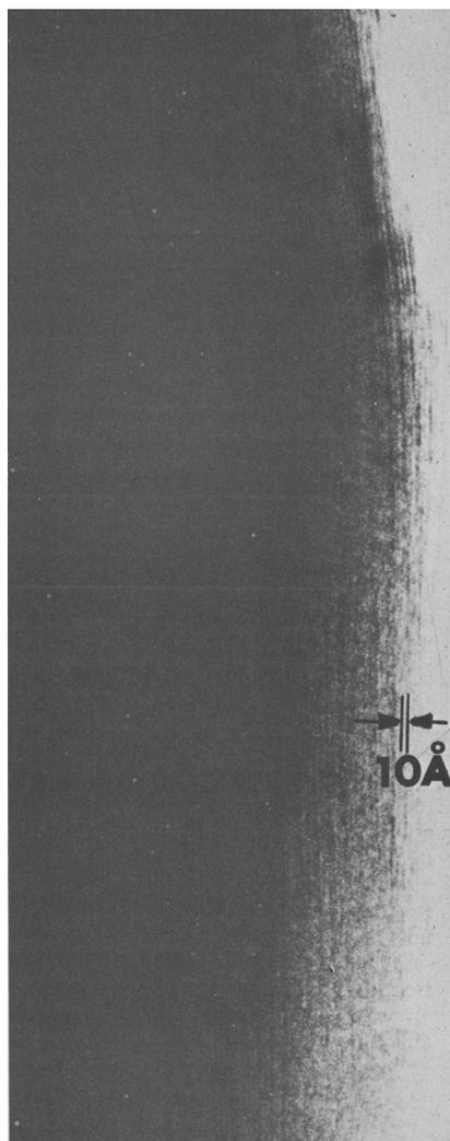
Fig. 4. An example of electron micrograph of layers showing the layer structure in which unexpanded layers are a major component.
