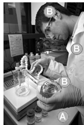
Fig. 1.2 BSL-1 type open workplace and personal protective equipment (PPE).
