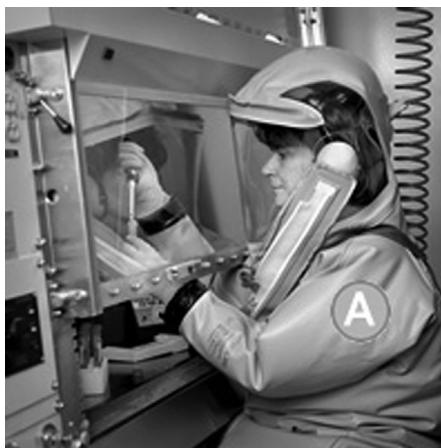
Fig. 1.5 BSL-4 workplace - note positive pressure body suit (PPE) in a Class III BSC.
