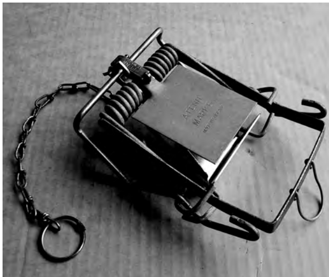
Fenn trap set showing the two striking bars: a rectangular bar on the right with thumb loop for setting and a cylindrical (rod-shaped) bar on left (set under trap dog and safety catch).
