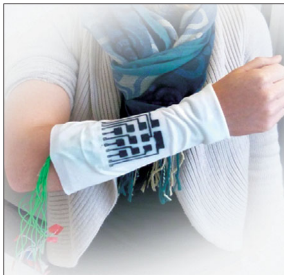
Wearable stretchable keyboard based on conducting polymer electrodes on knitted textile. Credit: Advanced Materials .
