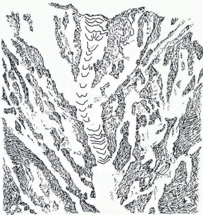
Fig. 9. The motion of the avalanche front, obtained from video films for the artificially released avalanche on 1 February 1988. Numbers correspond to those in Figure 10.
