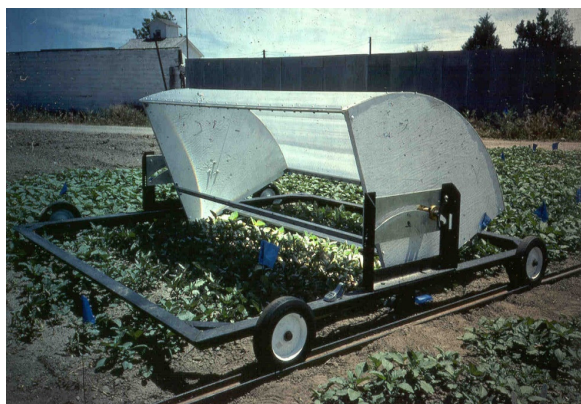
Figure 4. A Fresnel lens focuses sunlight to create a high temperature (>300 C) band for controlling weed seedlings (Johnson et al. 1990).
