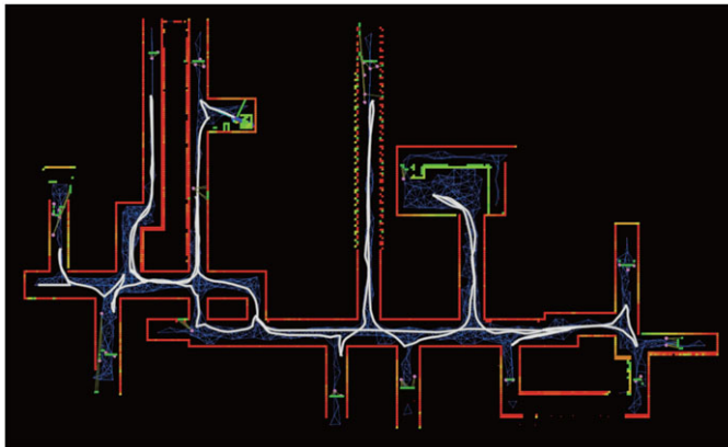
Figure 10. Exploration result of the indoor environment. The white lines denote the trajectories of the robot. It shows that the FAEL method exhibits limitations in fully exploring the highly convoluted environment.
