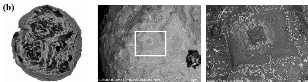
Figure 2. (a) OM of a typical barred olivine MM with a table of EDS-measured elemental composition by weight % [1] that indicates chondritic composition when compared by element/Si ratios to MMs obtained from the Antarctic [3]. (b) OM of a ~700 μm porphyritic olivine MM found at Nesodden, Akershus, Norway, with BSE micrographs indicating dendritic magnetite formation (bright features).
