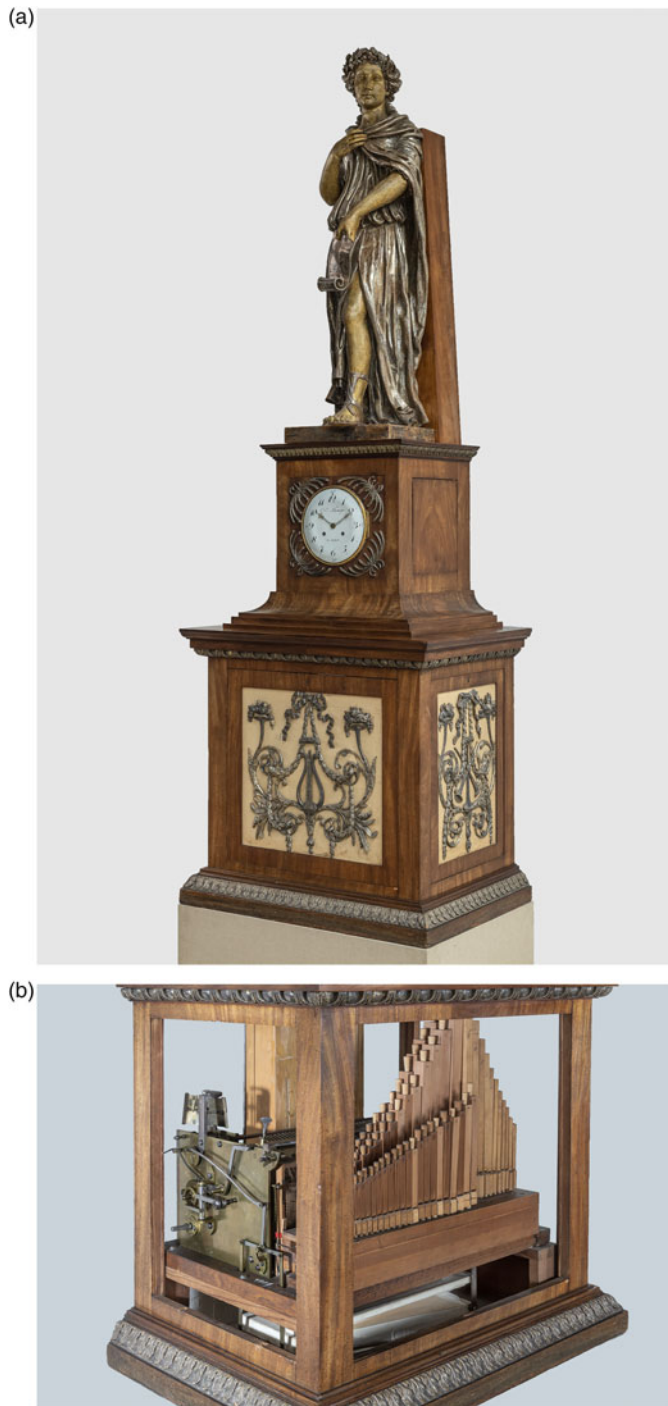
Figure 1. (a) A Flötenuhr by Christian Ernst Kleemeyer, dated 1775–1785; (b) the clockwork mechanism and pipes hidden inside its pedestal. Photos by Oliver Ziebe, 2022. Courtesy of the Musikinstrumenten-Museum, Staatliches Institut für Musikforschung SPK Berlin (object no. 4901)
