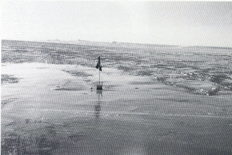
Fig. 7. Icing at stake 50, photographed on 10 January. The stake is 1.05 m high. This smooth surface later started to develop into an ablation crust as can be seen outside the icing area.
