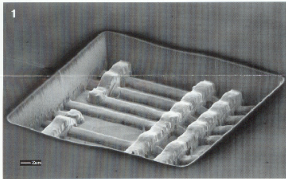
FIG. 3 Water enhanced etch to expose metal lines under polyimide
