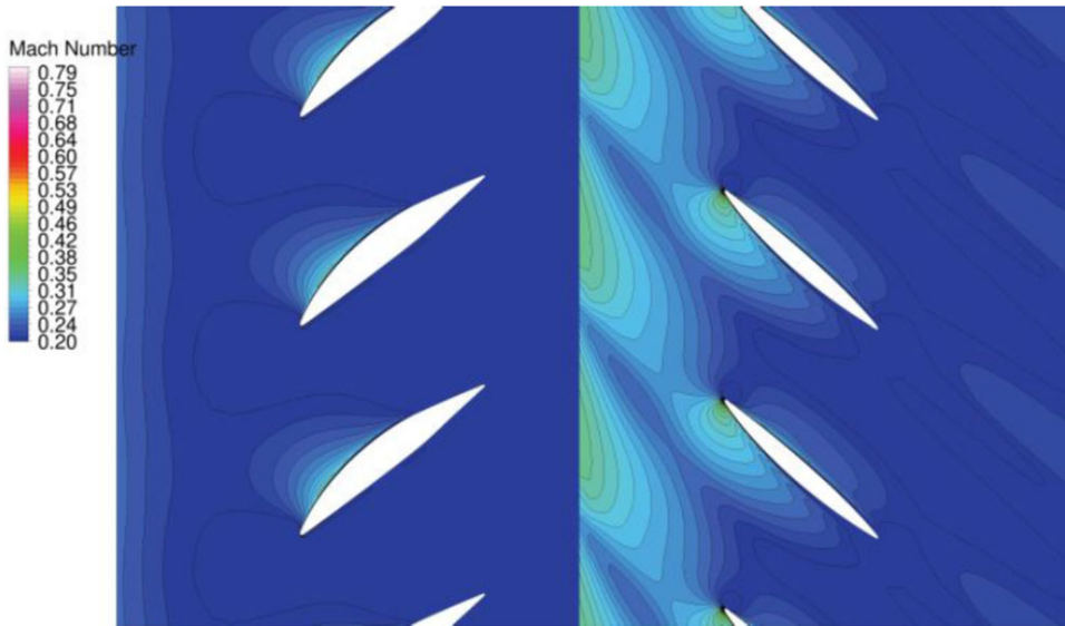
Figure 5. Mach number at 10% blade span in blade-to-blade representation.
