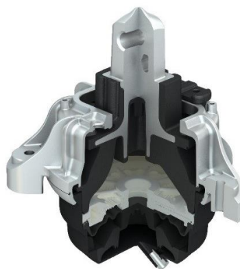
Figure 2. Hydraulic vehicle engine mount (Königs and Zimmermann, 2016)
