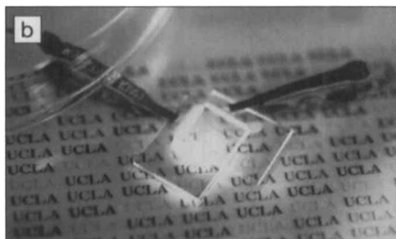
Transparent solution light-emitting device (SLED). (a) An unbiased transparent SLED; (b) a biased transparent SLED.
