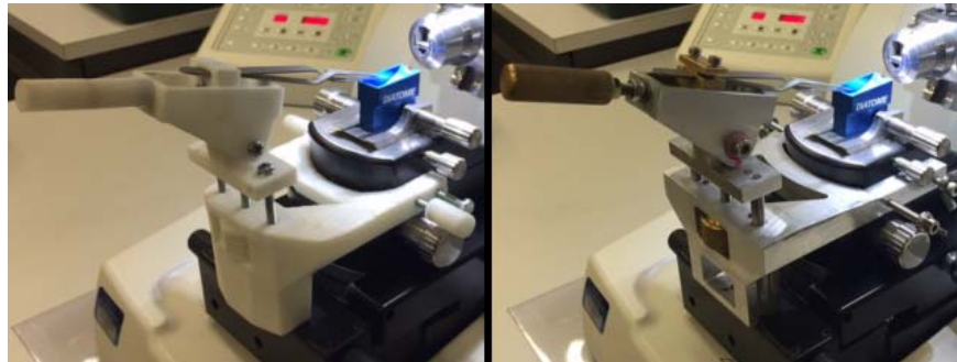
Figure 2: Left, 3D printed version install on a Leica UC7, the design should be compatible with several brand sof ultramicrotome. Right, CNC machined version of the tool on the UC7.
