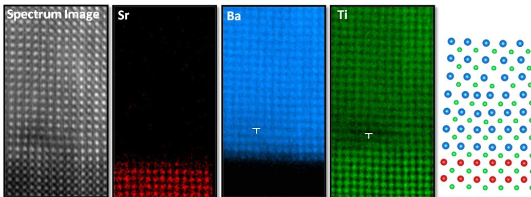
**Figure 2.** Elemental EELS mapping for BaTiO<sub>3</sub>/SrTiO<sub>3</sub> heterostructure with misfit dislocation, confirming no inter-layer diffusion, together with the proposed structural model. The core-less energies for elemental mapping were Sr L<sub>2,3</sub> (1940 eV; 2007 eV), Ti L<sub>2,3</sub> (456 eV, 462 eV), Ba M<sub>4,5</sub> (781 eV, 796 eV), and O K (532 eV).
