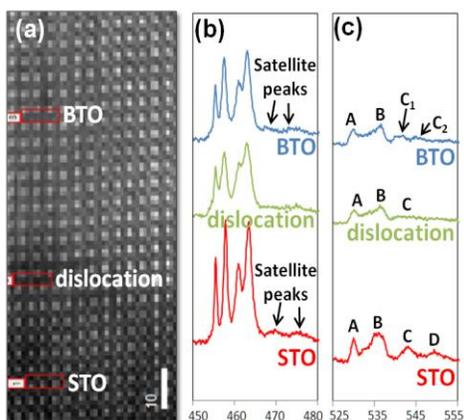
**Figure 3.** (a) HAADF image of BTO/STO heterostructure. Corresponding electron-energy-loss near-edge structure for (b) Ti L<sub>2,3</sub>, and (c) O K edges, for STO substrate, dislocation, and BTO film, as indicated. The core-less energies used for mapping were Ti L<sub>2,3</sub> (456 eV, 462 eV), and O K (532 eV), as indicated.
