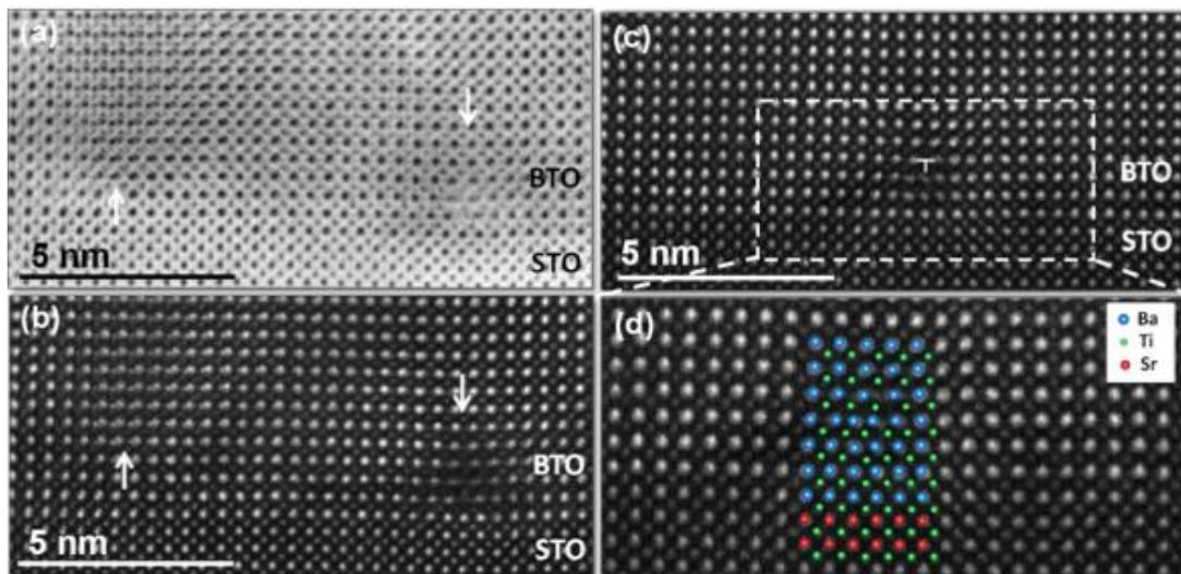
**Figure 1.** (a) LABF, and (b) HAADF, images showing BaTiO<sub>3</sub>/SrTiO<sub>3</sub> heterostructure with misfit dislocation and anti-phase boundaries. (c) HAADF image of BaTiO<sub>3</sub>/SrTiO<sub>3</sub> misfit dislocation with different offset from interface. (d) enlargement of dislocation core in (c) with proposed crystal structure.
