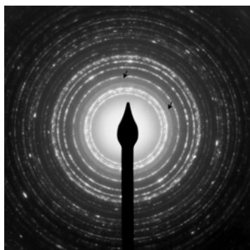
Fig. 1 Representative diffraction pattern from Pt-ZnO catalysts.
