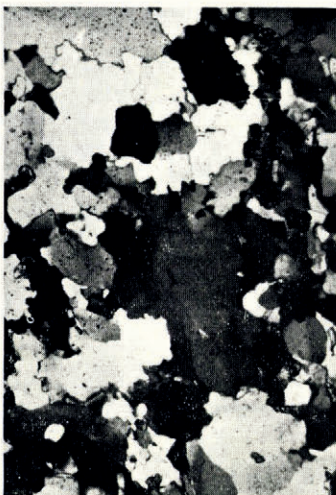
Fig. 1 (top left). Tessellate quartz-mosaic of psammitic granulite, east of Beinn nan Losgann, Ardnamurchan. Mosaic largely quartz, with sporadic alkali feldspar and mica. Nicols crossed. \times 32 . Compare Fig. 2
