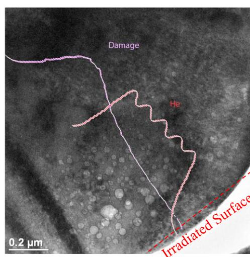
**Figure 1.**  $\text{Fe}^{++}$  irradiation damage curve and implanted helium distributed superimposed over sample irradiated to 375 dpa at 480°C with a dose rate of  $5.4 \times 10^{-4}$  dpa/s.
