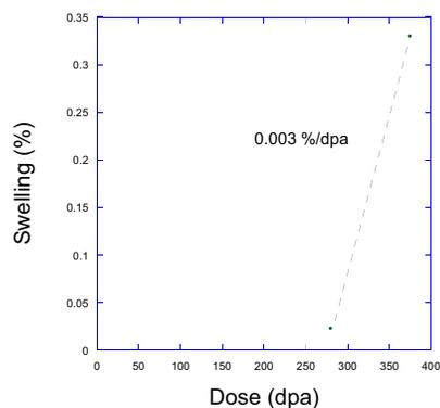
**Figure 3.** Swelling versus dose in irradiated T91 at 440°C
