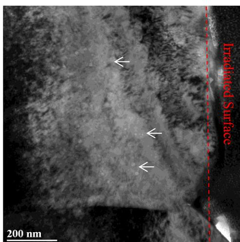
**Figure 2.** T91 irradiated to 280 dpa at 440°C and at  $7.92 \times 10^{-4}$  dpa/s. Selected voids marked with white arrows.
