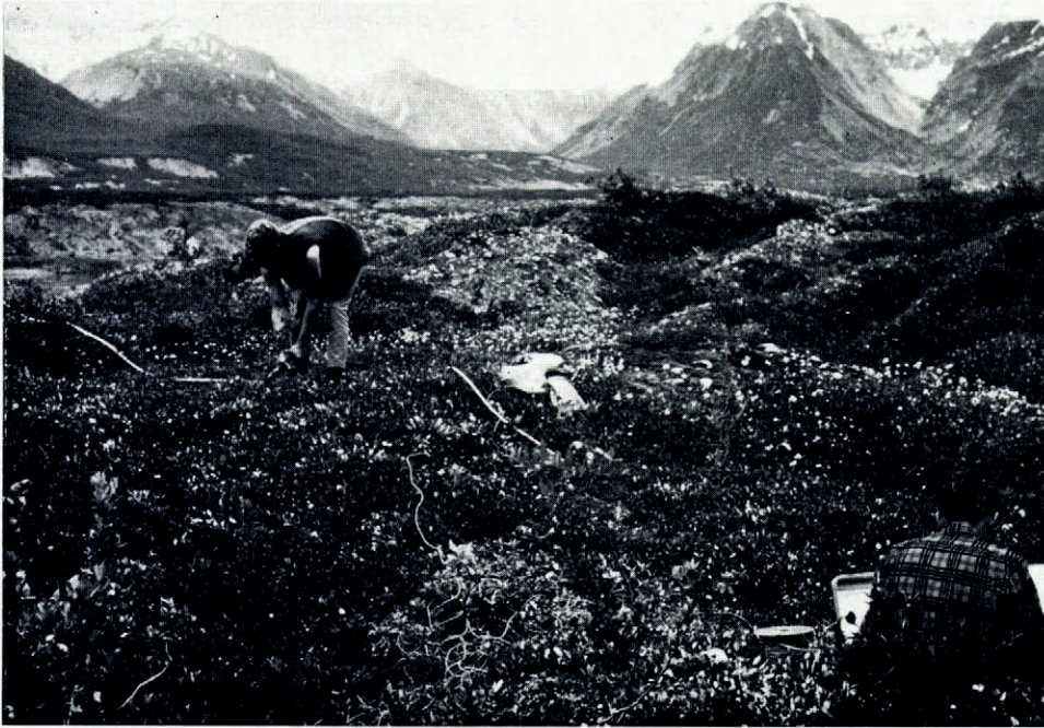
Fig. 4. Hummocky vegetated surface of kame terrace. Hammer seismograph is in operation to determine depth to stagnant ice. View is north-east.
