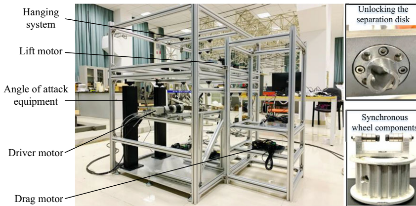
Figure 12. Pneumatic load simulation test platform.
