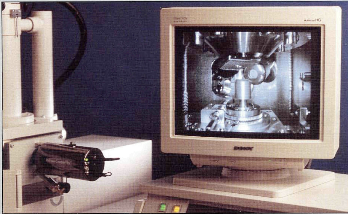
ETP Chamber View mounted on SEM with SEM chamber image
