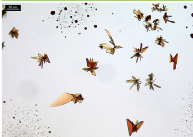
Figure 1. 1 PPP of codeine and 10 µL of reagent. Crystals form rosettes of triangles and hatchet blades.
