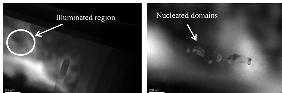
Figure 3. A. Image of monodomain area. Circle shows illuminated area. B. Domains which were locally nucleated due to the condensed beam. Nucleation occurred at perimeter of beam, shown in 3A.
