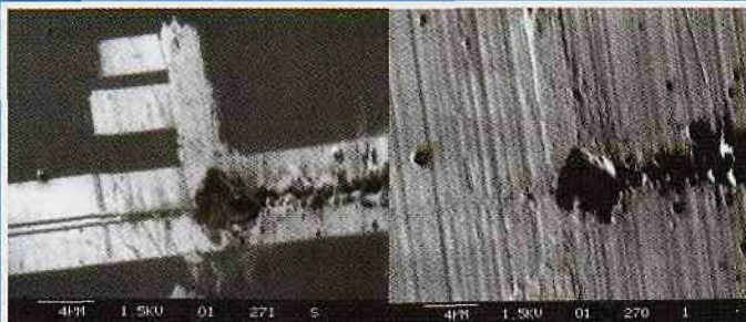
Figure 3. Uncoated recording head tilted by 45deg. to the low-loss electron (LLE) detector on the left.(5) Beam energy = 1.5 keV to minimise charging: (a) SE image. (b) LLE image from the same field of view. Energy window = 500 eV. Field of view measures 30 micrometers left to right.
