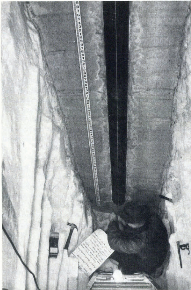
Fig. 2. Looking down into a snow pit that was excavated with the use of an electric chain saw. The pit was excavated to reveal the snow displacement along a 6 in [0.15 m] diameter, close-ended pipe pile driven into \sim 0.54 \text{ Mg m}^{-3} density snow. After planing the pit wall smooth and then dyeing the surface, the natural stratigraphic layering became visible.
