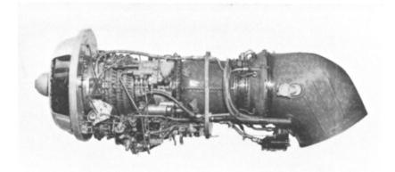
General Electric is available in the Gnome, and the de Havilland Engine Company will be type-testing the uprated version of the engine, designated the Gnome H1200, towards the end of 1960
