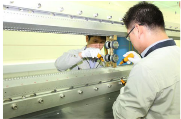
Figure 14. Prototype HX undulator undergoing the pole tuning procedure.
