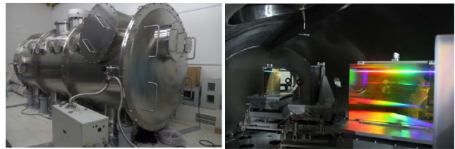
Figure 13. Compressor tank (left) and an inner image of the gold-coated gratings (right).
