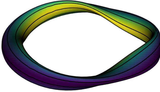
FIGURE 1. Plasma boundary of a quasisymmetric stellarator with three field periods, n_{fp} = 3 . The colours represent the magnetic field strength at the boundary and a magnetic field line is shown in black.
