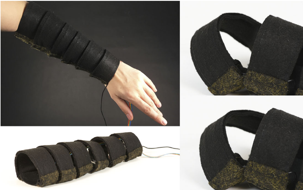
Figure 2. A prototype of an affective sleeve, used in prior study, made from felt fabric and a shape memory alloy (nitinol). When electrical current passed through the nitinol wires of a sleeve's cuff, the cuff changed shape producing slight warmth and pressure. Developed by the author and collaborators (Papadopoulou et al. 2019).
