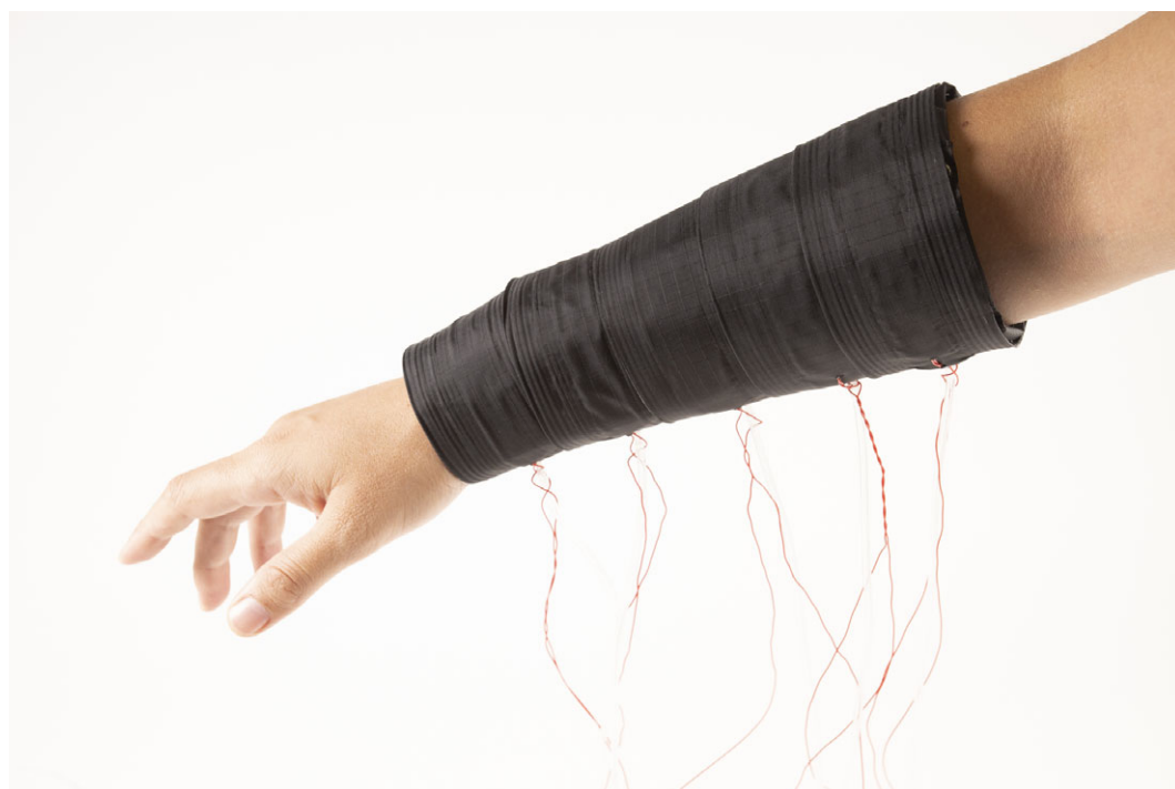
Figure 6. Close-up photograph of the prototype of the pneumatic affective sleeve used in the study.
