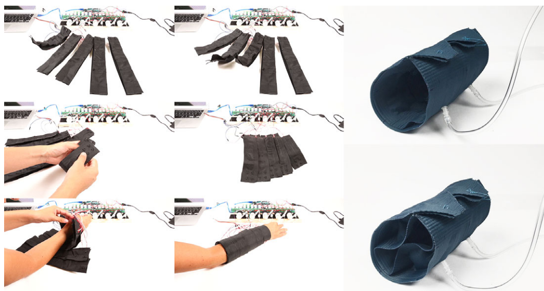
Figure 5. The pneumatic affective sleeve was comprised of five cuffs that curved around the arm upon pressurization and also included embedded heatpads. The sleeve was designed to be modular to accommodate different body sizes (left). Preliminary prototype of the pneumatic affective sleeve showing how the novel material mechanism forces the air towards the skin increasing felt pressure and eliminating any ballooning effects (right).
